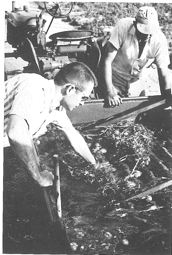
The machine in photo above was built to harvest tomatoes for the processing industry. It was found unsuitable for fresh market tomatoes. At right, W. W. Deen, Jr., of the Everglades Experiment Station, tests a principle which might work for handling fresh tomatoes.
