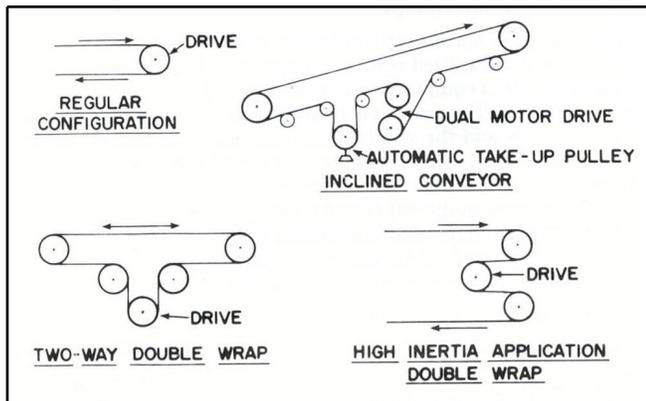
Figure 15. Various belt drive configurations.
