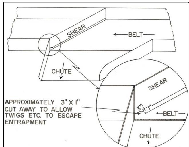
**Figure 14.** Self-cleaning shear.
