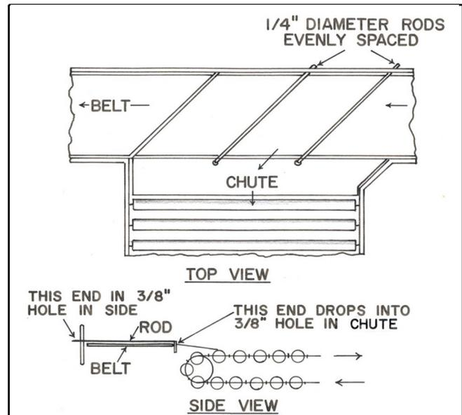
**Figure 13.** Use of diversion rods with a fixed shear. The rods are NOT fixed in place. They are inserted through holes in the chute and the side of the conveyor and ride on the surface of the belt.
