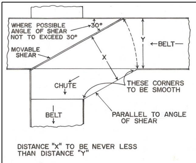
**Figure 11.** Cutting back the inside corner of a sheared turn. A shear angle of 30° is optimum, but 40° can be used. A supporting plate that prevents the belt from sagging under the shear helps to minimize the change of fruit injury.
