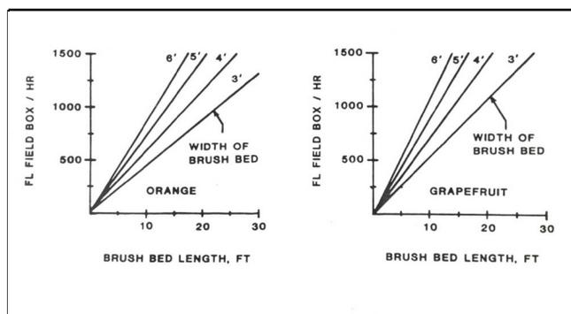
**Figure 4.** Brush bed capacities for oranges and grapefruit (30 second wash time).
