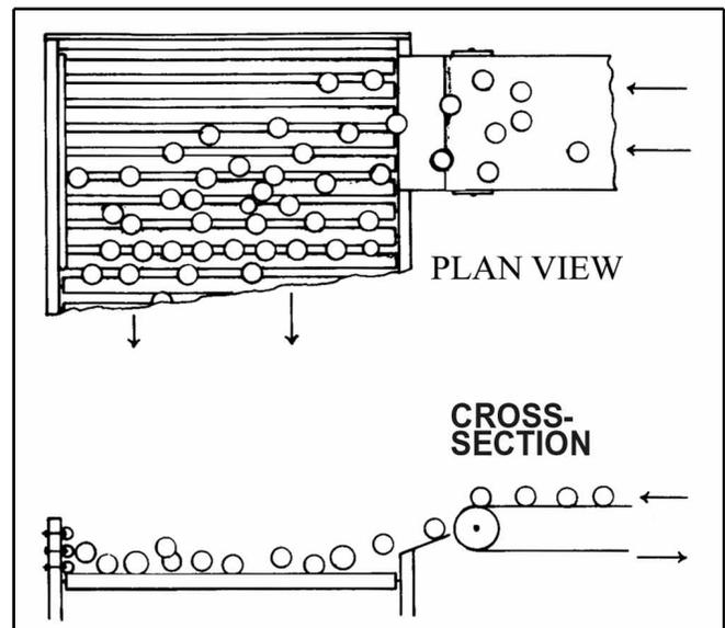
Figure 10. Over-the-end delivery for a right-angle turn onto a belt, roller conveyor, or slat conveyor. This method is preferable to the use of a shear. Triangular delivery chute is necessary when delivering onto a slat conveyor but not essential for either a belt or roller conveyor.
