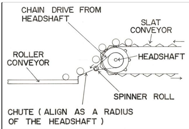
Figure 8. Spinner roll on a slat conveyor delivery.
