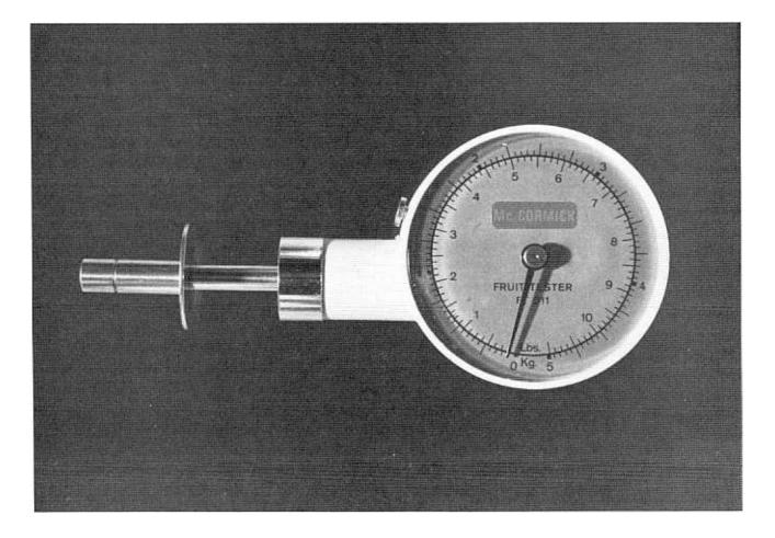
Figure 6. Fruit pressure tester. EFFEGI, Alfonsine, Italy
