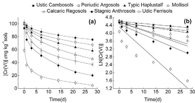
**Fig. 2.** Time courses for hexavalent chromium [Cr(VI)] after addition of 100 mg kg<sup>-1</sup> Cr(VI) to seven soils. (a) Dissolved Cr(VI). (b) First-order plots of ln[Cr(VI)]. The slope of the lines is equal to the first-order rate constant. Vertical scales are different.
