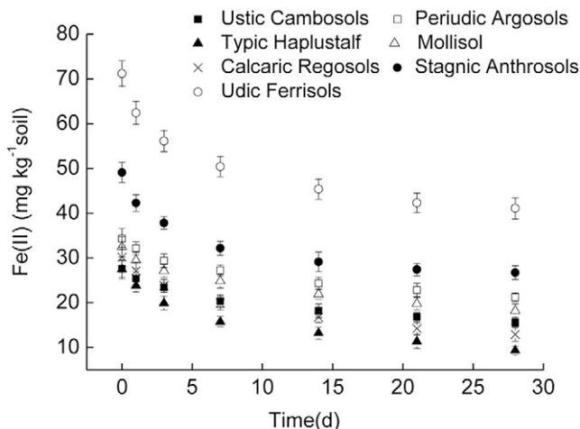
Fig. 3. Time courses for Fe(II) after addition of 100 mg kg<sup>-1</sup> hexavalent Cr to seven soils.
