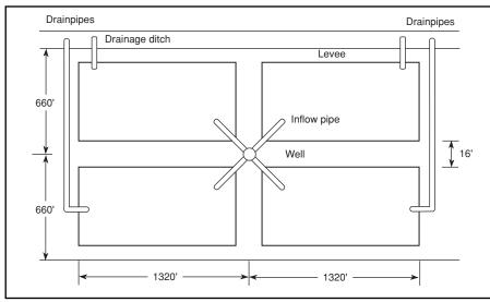
Figure 1. Layout of a typical levee-type catfish pond.
