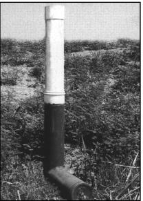
*Figure 3. Outside drain fitted with a "T-stand pipe" amd alfalfa valve.*
