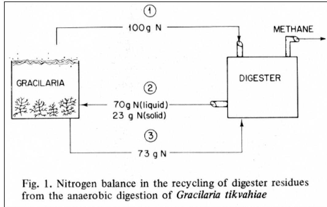
Fig. 1. Nitrogen balance in the recycling of digester residues from the anaerobic digestion of *Gracilaria tikvahiae*
