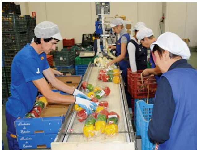
FIGURE 8.8 Greenhouse-grown bell pepper packed with polymeric film. The package extends fruit postharvest life by reducing fruit transpiration. The package also facilitates fruit handling and provides protection to reduce fruit mechanical damage. The package may help in marketing by allowing labeling and providing an appealing appearance of the fruit.
