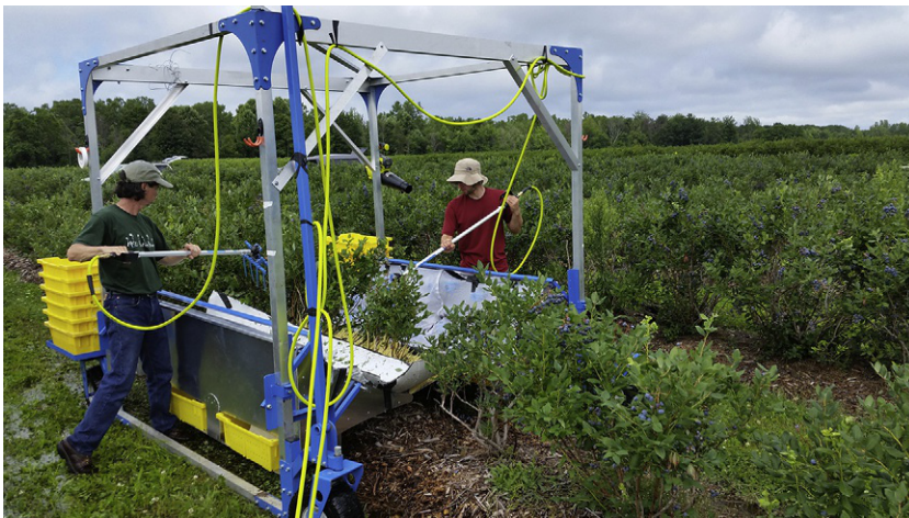
FIG. 5.18 Semimechanical harvester for blueberry fruit. (Courtesy of Fumiomi Takeda)
