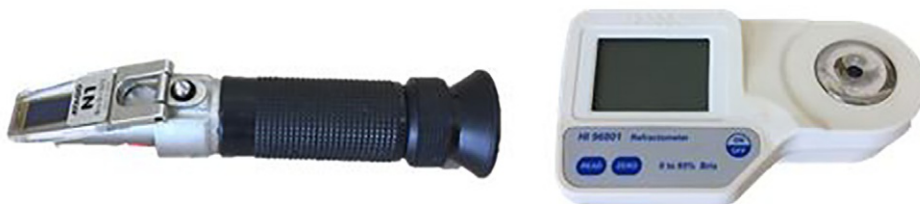
FIG. 5.8 Hand and digital refractometers.
