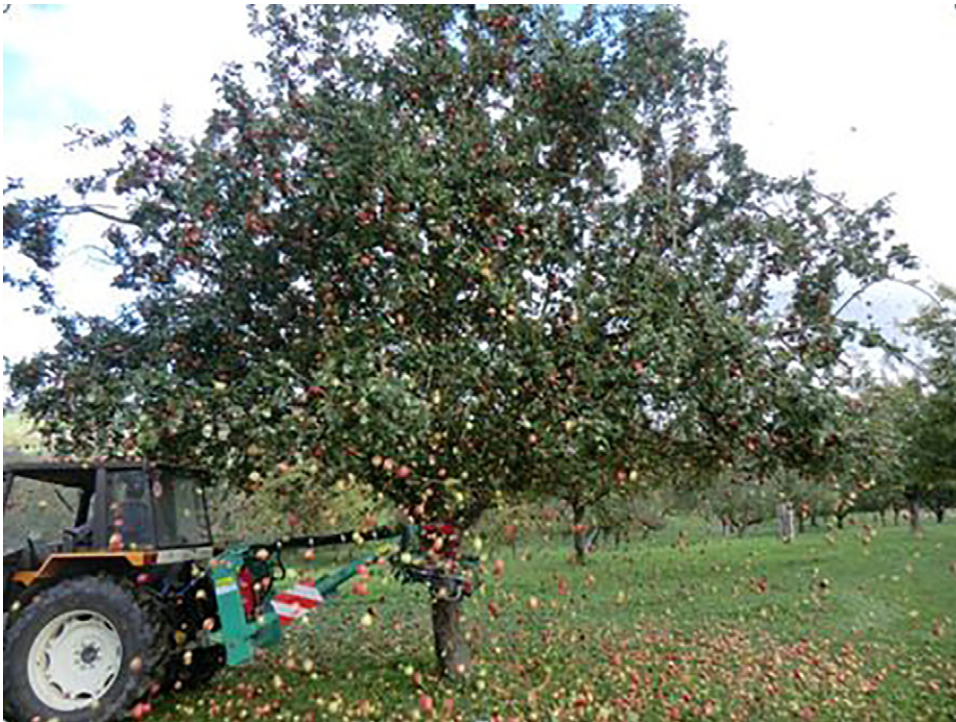
FIG. 5.19 Tractor-mounted trunk shaker for apples. Courtesy Feucht Obsttechnik GmbH Company.
