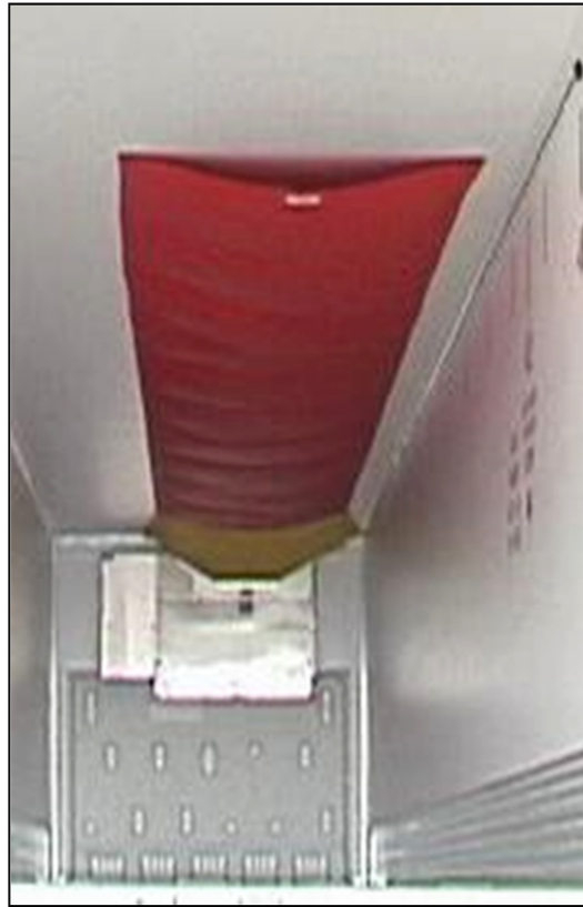
FIG. 18.9 Interior view of refrigerated trailer showing flat sidewalls, a duct extension, an air delivery chute attached to the ceiling of the reefer trailer, and the pressurized return air bulkhead. Source: Thermo King Corp.
