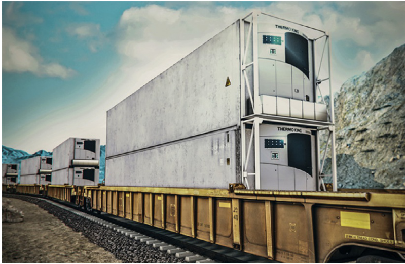
FIG. 18.7 Reefer containers double-stacked on rail flatcars. Source: From Thermo King Corp.
