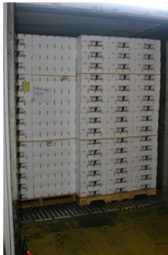
FIG. 18.20 Pictures of the correct stowing of palletized fruit in a bottom-air delivery reefer container. The upper picture shows initial stowage of pallets covering the floor with no vertical channels or gaps. The lower picture illustrates the rear of a load stowed with a 9' \times 11' pallet configuration. Sources: National Mango Board and PEB Commodities, Inc.
