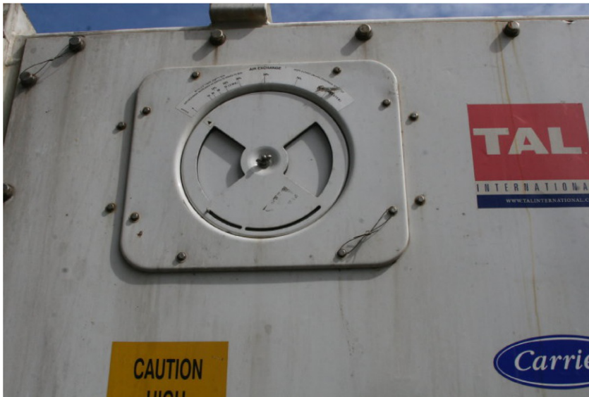
FIG. 18.4 Picture illustrating manual fresh air exchange within a reefer container. Source: PEB Commodities, Inc.
