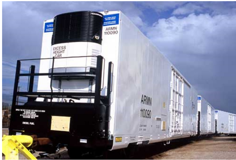
FIG. 18.11 External view of refrigerated railcar. Source: Thermo King Corp.
