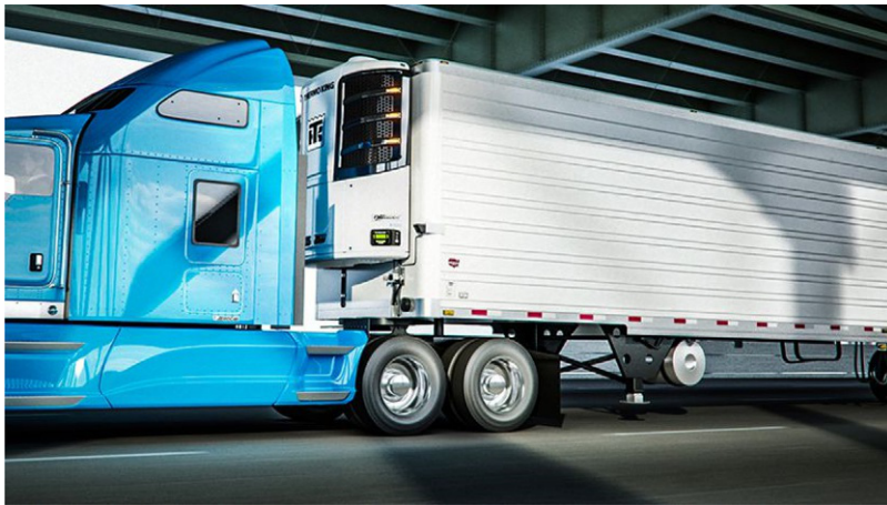
FIG. 18.8 External view of trailer, refrigeration unit and insulated trailer. Source: Thermo King Corp.
