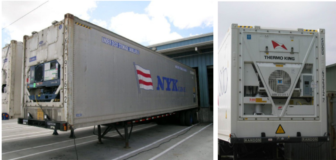
FIG. 18.2 External views of refrigerated containers showing an integral refrigeration unit attached to an insulated container (box) and a chassis. Source: PEB Commodities, Inc.
