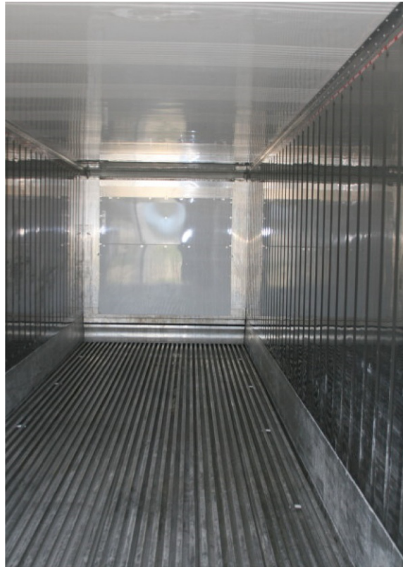
FIG. 18.3 Interior view of a refrigerated container showing corrugated sidewalls, "T" bar floor, return air register, and front bulkhead. Source: PEB Commodities, Inc.
