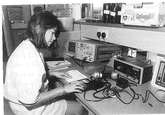
Figure 8 A colour difference meter being used to measure the colour of melons at Cranfield University in the United Kingdom. (Source: A.J. Hilton. Reproduced with permission of Cranfield University.)
