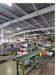
Using optical sorting with AI, they reduced from 220 people to 110. The machine takes around 100 pictures of the same tomato, 24 externals, and the rest infrared; it can detect around 3 thousand defects, different levels of severity, bruises, and scars.
