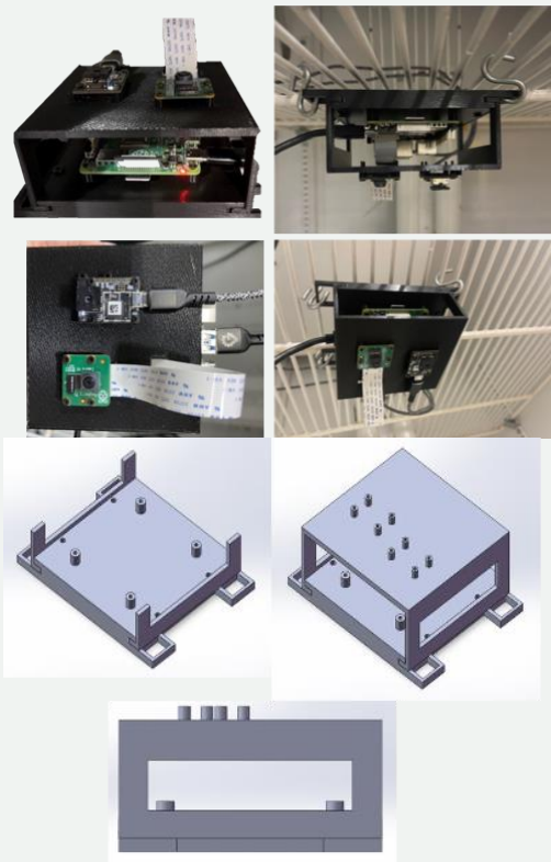
Figure 2. Construction of the camera module (left), 3D mockup design of the sensor housing (right).
