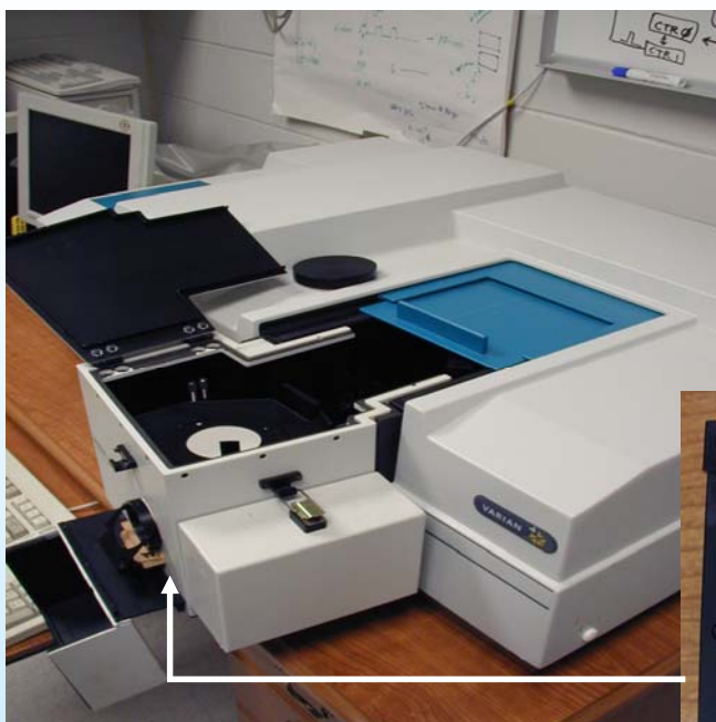
Spectrophotometer - Measures spectral reflectance from 200nm to 2500nm
