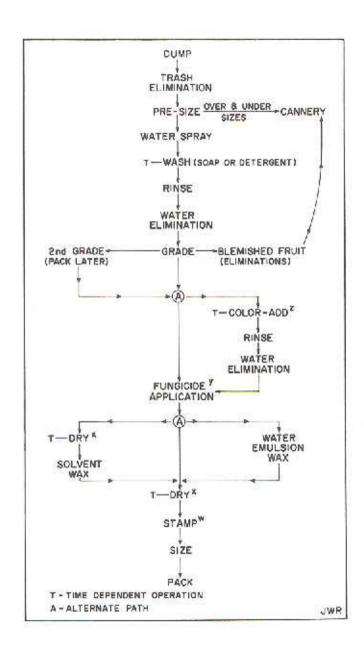
Figure 1. Unit operations in typical Florida citrus packinghouse (6).
