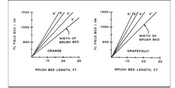
**Figure 4.** Brush bed capacities for oranges and grapefruit (30 second wash time).
