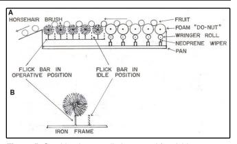
**Figure 5.** Combined water-eliminator and fungicide-wax applicator. A. Major components of the unit: sponge rubber rolls with wringer rolls wiped by neoprene wipers constitute the water-eliminator section; horsehair brushes with flick bars follow as a brushbed for application of water-emulsion wax or fungicide. Note that flick bars are moved manually and only in contact position when rinsing the brushes. B. Flick bar detail.
