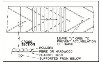
**Figure 3.** Angled supports under roller conveyors. Spacing is such that every roller is supported by at least two supports at all times, wear is distributed evenly over whole length of each roller, and the rollers are partially self-cleaning.
