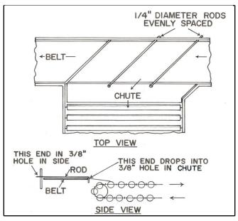
**Figure 13.** Use of diversion rods with a fixed shear. The rods are NOT fixed in place. They are inserted through holes in the chute and the side of the conveyor and ride on the surface of the belt.
