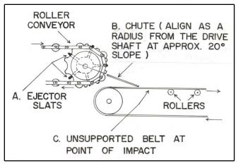
**Figure 7.** Delivery from roller conveyor to a belt. A. Ejector slats. B. Chute aligned as the radius of the head shaft. C. Delivery onto unsupported belt where one roller has been removed.
