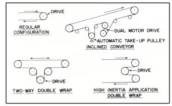
Figure 15. Various belt drive configurations.
