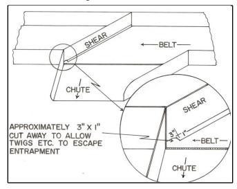
Figure 14. Self-cleaning shear.
