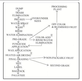
**Figure 1.** Logical order for a packingline when only one grade is packed most of the time. Degreening and frozen fruit separation are not included here, being covered in separate publications (25, 26). T denotes time-dependent operation.
