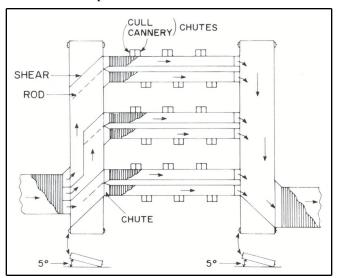
**Figure 6.** Multiple grade tables. By contrast with a single long grading table, the stream of fruit divides into three standard width graders, speed of forward travel is slowed to one-third and each fruit is examined by one-third as many graders as diagramed for an installation with three two-sided grading tables.
