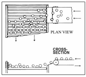
**Figure 10.** Over-the-end delivery for a right-angle turn onto a belt, roller conveyor, or slat conveyor. This method is preferable to the use of a shear. Triangular delivery chute is necessary when delivering onto a slat conveyor but not essential for either a belt or roller conveyor.
