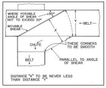
**Figure 11.** Cutting back the inside corner of a sheared turn. A shear angle of  $30^{\circ}$  is optimum, but  $40^{\circ}$  can be used. A supporting plate that prevents the belt from sagging under the shear helps to minimize the change of fruit injury.
