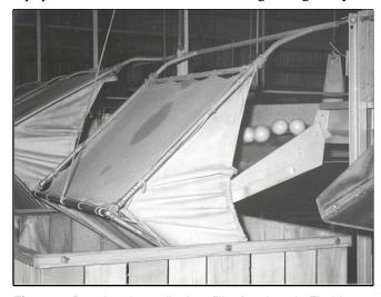
**Figure 2.** Deceleration pallet box filler for citrus in Florida. Counter-weighted devices begin low in the pallet box and are gradually raised manually as the box fills. There are two pallet boxes per fruit size to allow ample time to remove a full box and replace it with an empty box without interrupting the fruit flow.
