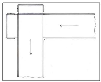
**Figure 12.** When conveying fruit on two belts at the same elevation, the second belt should be on top. Over-the-end delivery (Fig. 10) is preferred.
