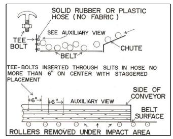
**Figure 9.** Solid rubber or plastic hose (no incorporated fabric) used as a bumper opposite a right-angle delivery.
